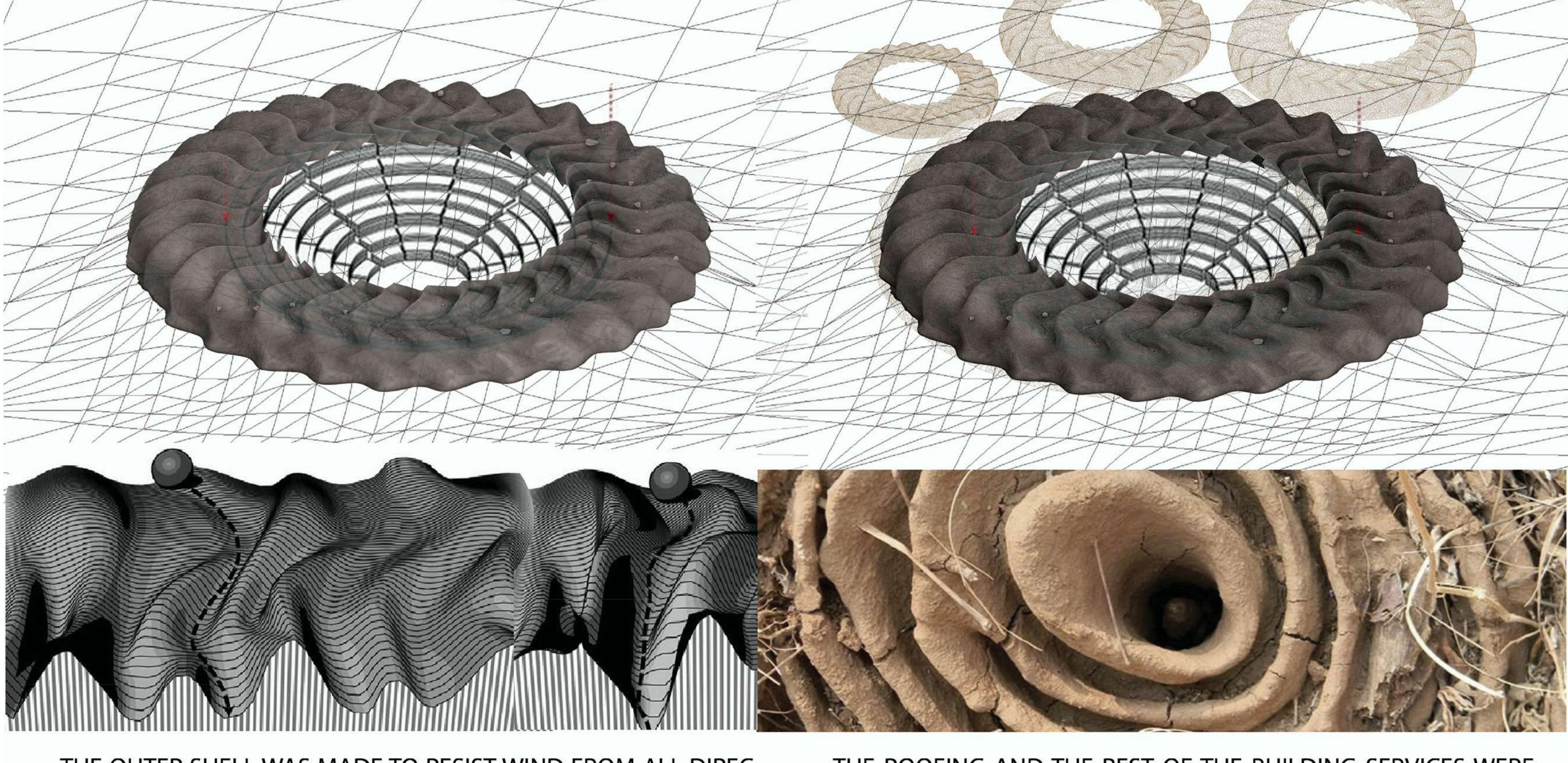
THE OUTER SHELL WAS MADE TO RESIST WIND FROM ALL DIREC-TIONS AND TO MATCH THE SHAPE OF THE SURROUNDING ENVI-RONMENT
